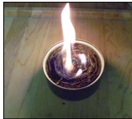
A buddy burner, made from a tuna can, cardboard and wax.
