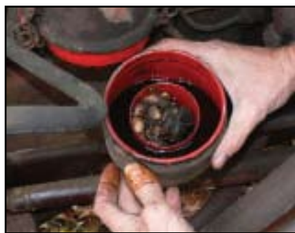
Above: Many engines use an oil bath air filter. You should check the oil level twice a year, and clean out the gunk. Below: Apparently a mouse has been storing acorns in Henry's air filter! I have no idea how he managed to get them in there.
